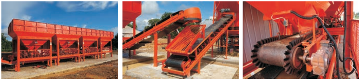
Side wall type belt conveyor / Alarm sensor / Direct connection
